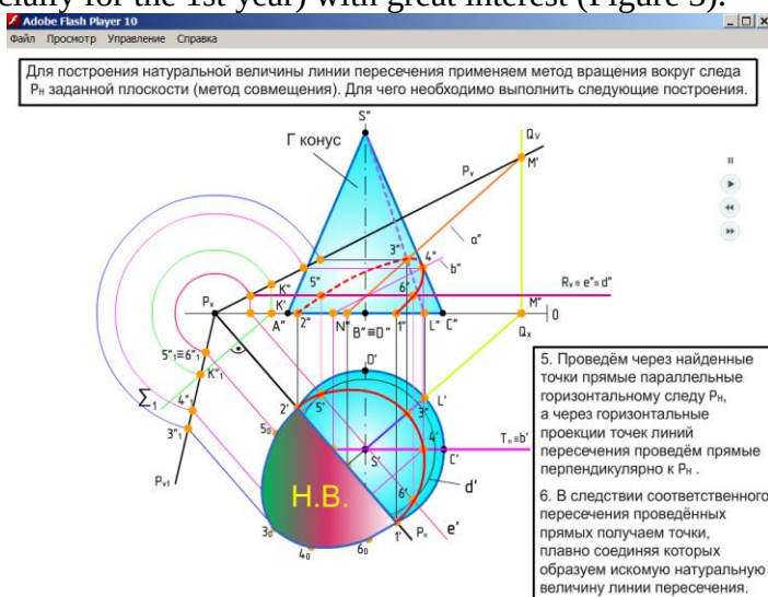
Figure 3 - Fragment of an animation clip on constructing the intersection line of a plane with a cone using the Flash program
